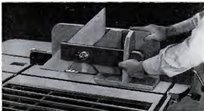
When cutting tenons or grooving ends of stock mitered at 45 deg., backstop is removed. Photo above shows first grooving operation for spline
